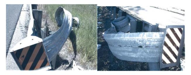
93. Harman's presentation demonstrated how Trinity's undisclosed modifications were in fact preventing the ET-Plus from accomplishing this core task. Harman had uncovered numerous examples of failed ET-Plus heads, which – as he documented in gruesome detail – transformed guardrails into deadly spears that entered the passenger cabin of the vehicles, causing catastrophic injuries to their passengers:
